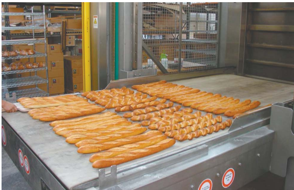
Product baked in a WP Matador MDV 220 with a WP OberJunior loading system..
